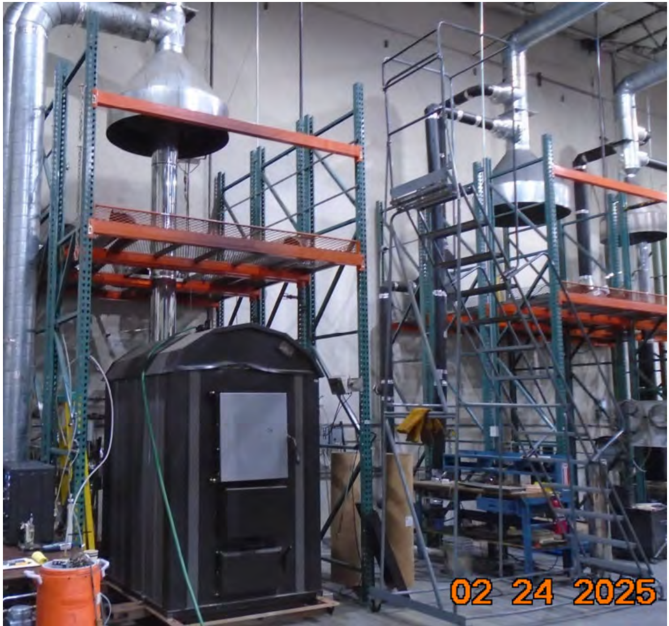
Figure 7 - Central Boiler Classic Edge 760.1 installed in test structure and general work area
