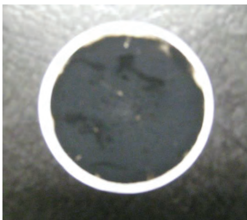
Figure 20 - Effective facial area of sample filter (file photo, not from the evaluation in this report)
